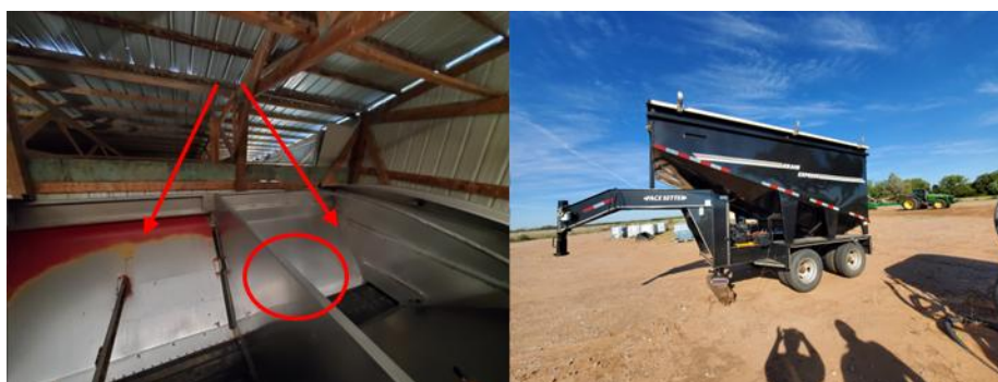
Figure 6. Equipment purchased to implement cover crops. Note the double load out in the trailer on the left to carry different cover crops (the red circle shows the divider in the trailer). The cover crops are spread during / after harvest. Photo credit: P. Cunningham
