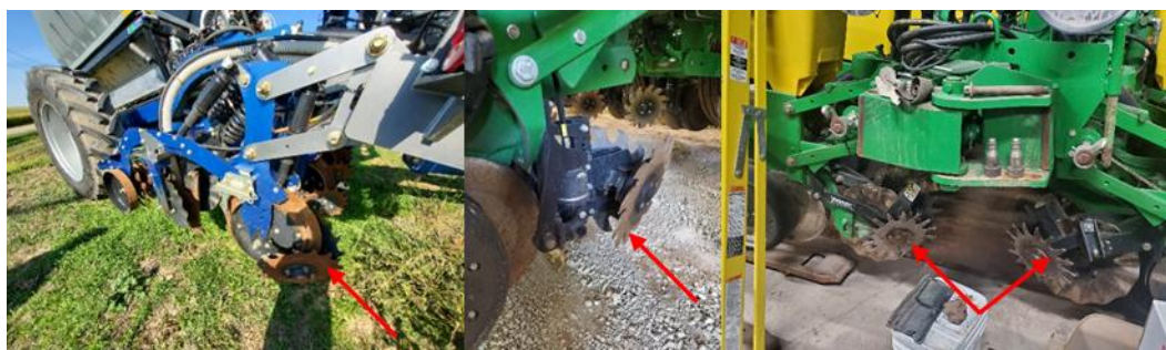
Figure 5. Equipment purchased to implement low impact tilling / no-till. Note the choppers at the back of equipment to assist in knocking down residue from the prior years' crops. When reduced tillage is implemented, residue must be managed due to the lack of conventional tillage and chopping. Photo credit: P. Cunningham
