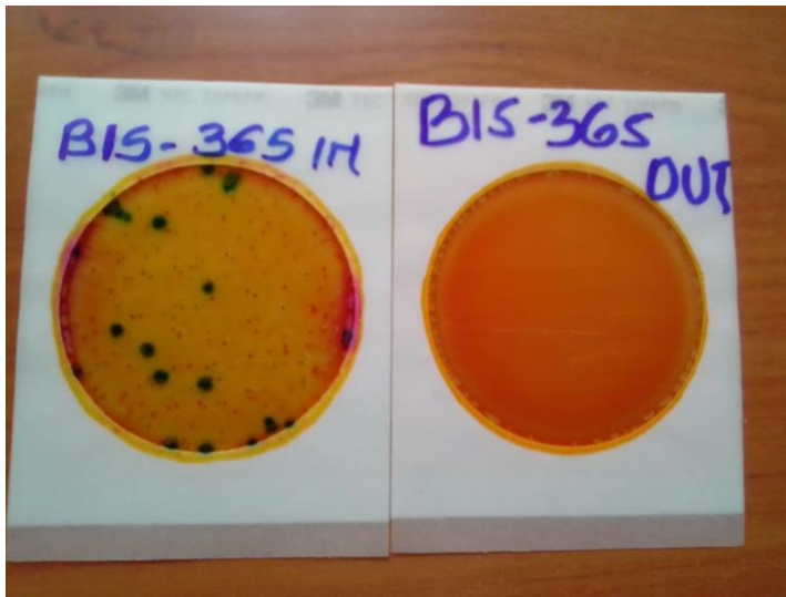
Figure 9: Diagram showing presence and absence of E. coli for a BSF user.
