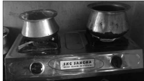
Biogas stoves provided by SKGS along with the biodigester unit.
