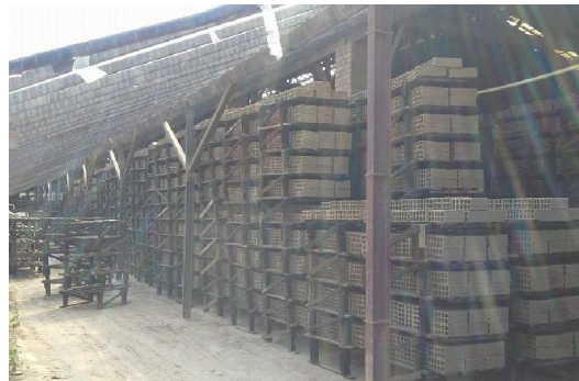
Figure 8: Natural sheltered drying process of ceramic pieces at Vulcão Ceramic.
