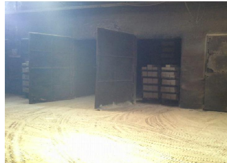
Figure 7: Artificial drying process of ceramic pieces at Vulcão Ceramic.
