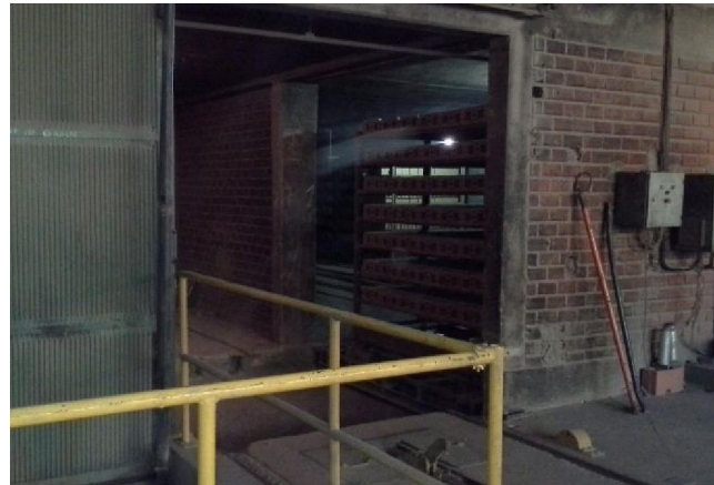
Figure 2: Continuous artificial process for ceramic drying at Argibem Ceramic.
