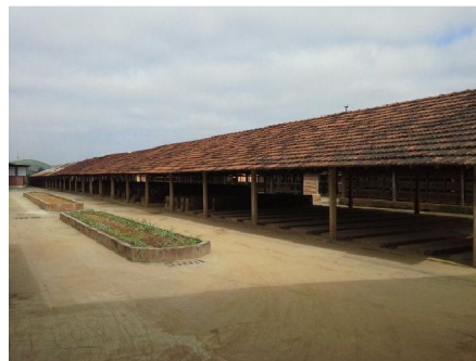
Figure 4: Natural drying process of ceramic pieces at São Sebastião Ceramic.
