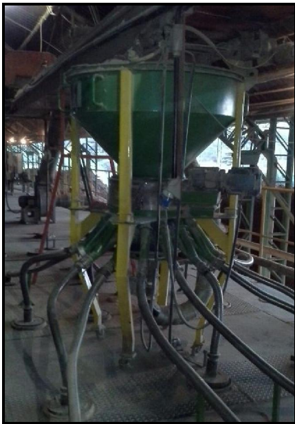
Figure 1: Automatic biomass feeding machine at Argibem Ceramic.
