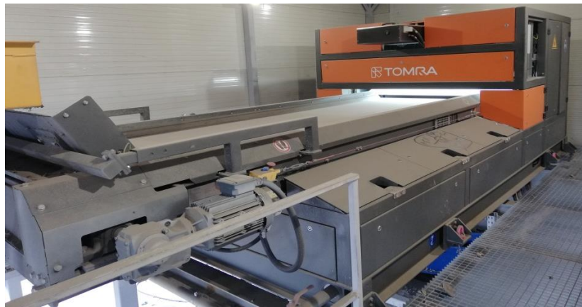
Picture 26: TOMRA COMBISENS machine – optical sorting installation
