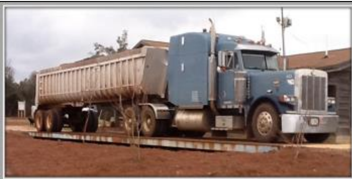
Stage 1: Weighing of loaded truck containing waste in weigh bridge scale
