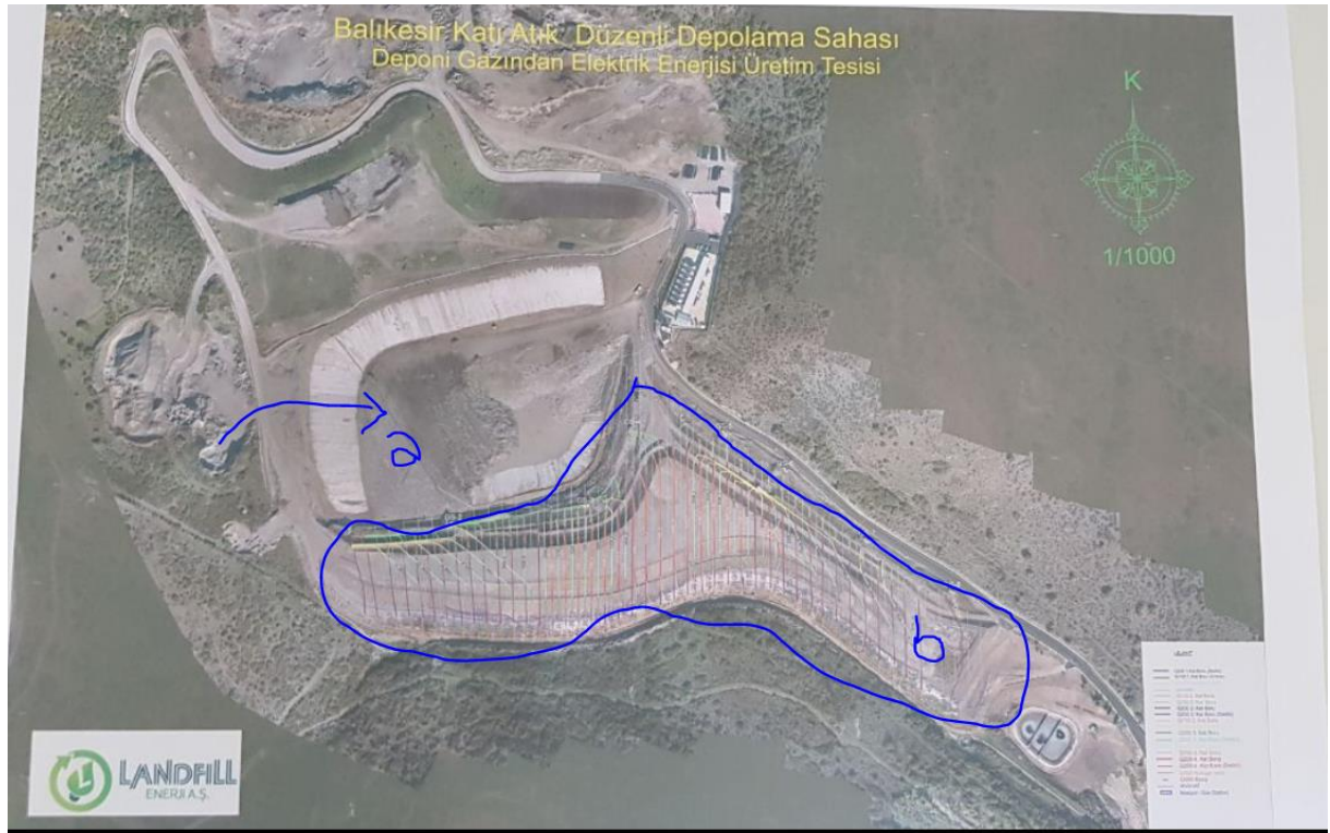
Figure 2. Landfill Gas collection areas. Section a. area expansion for more waste depositing. Section b. Old waste deposition area (2005-2021)
