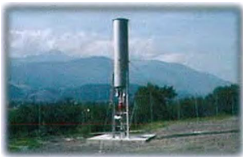
Figure 1.6. Torch/Flare system (Example)
