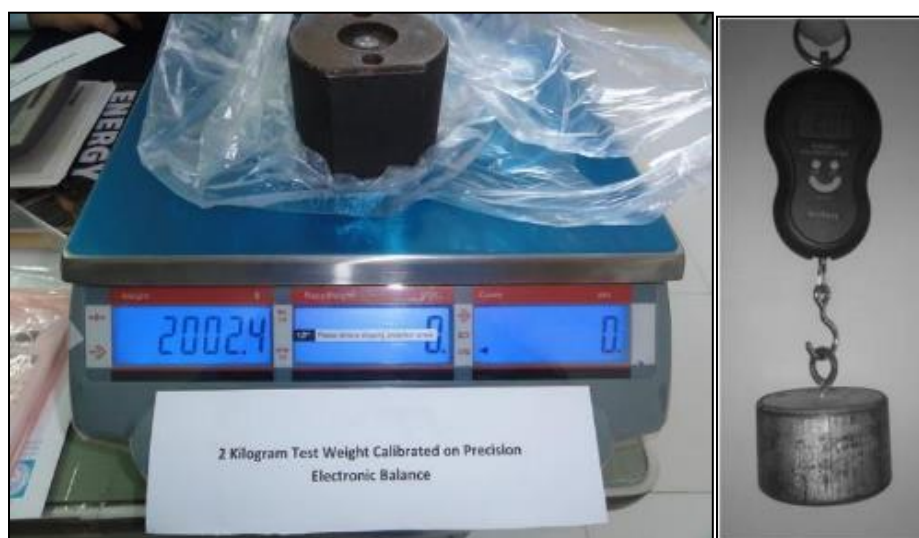
Figure 5: Weight check on Electronic Balance and the electronic Newton scale
