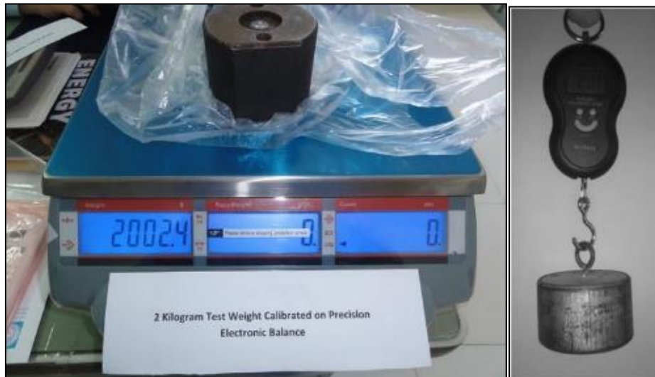
Figure 3: Weight check on Electronic Balance and the electronic Newton scale
