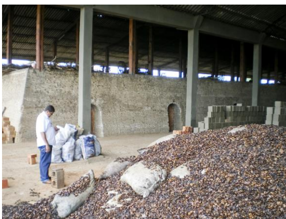
Figure 03. Cashew nut shells stored prior to use as fuel in Ceagra Ceramic.
