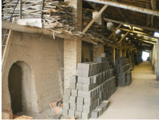
Figure 1. Hoffmann kiln being fed with renewable biomass in Antônio Ceramic.
