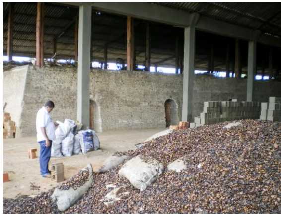
Figure 6. Cashew nut shells stored prior to use as fuel in Ceagra Ceramic.
