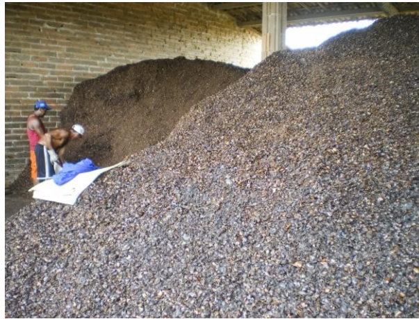
Figure 2. Cashew nut shells stored prior to use as fuel in Antônio Ceramic.
