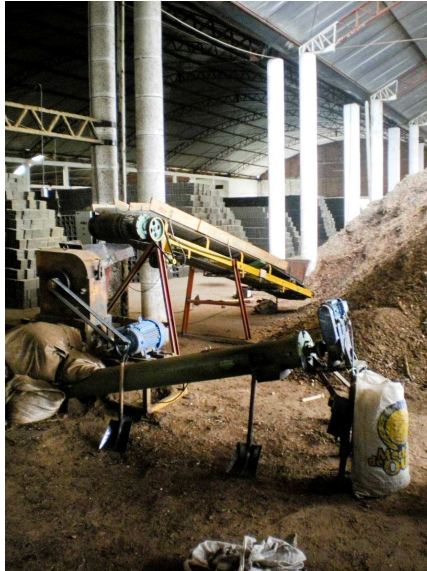
Figure 05. Biomass being processed to be used as fuel in Eliane Ceramic.
