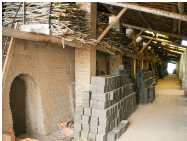
Figure 02. Hoffmann kiln being fed with renewable biomass in Antônio Ceramic.
