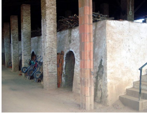
Figure 9. Hoffmann kiln being fed with renewable biomass in Santa Rita Ceramic.
