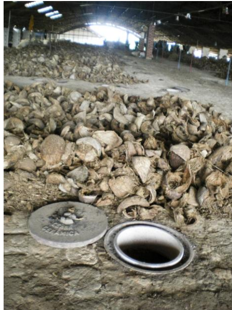
Figure 7. Hoffmann kiln being fed with renewable biomass (coconut residues) in Eliane Ceramic.
