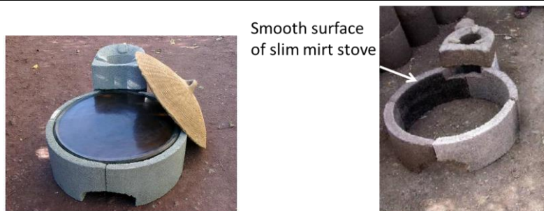
Figure 2: Mirt stove with baking plate ("mitad") and cover 4 and slim Mirt without baking plate 5
