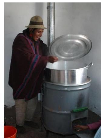
CEDESOL Rocket stove for institutional and commercial application.
