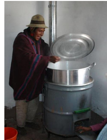
CEDESOL Rocket stove for institutional and commercial application.
