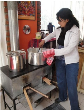
CEDESOL Rocket stove for domestic application
