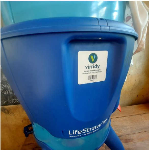
Figure 4. Example of the barcode with the unique ID number of the filter
