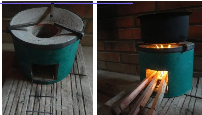
Figure 1: Efficient Stove Design (Gabanyibicanwa Stove)
