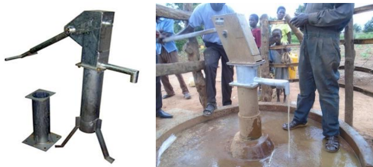
An example of a U3 modified pump in action, from a well maintained waterpoint.
