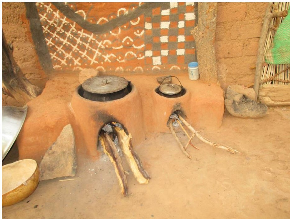
Locally produced efficient F3PA cookstove
