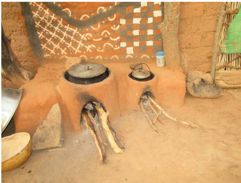
Locally produced efficient F3PA cookstove
