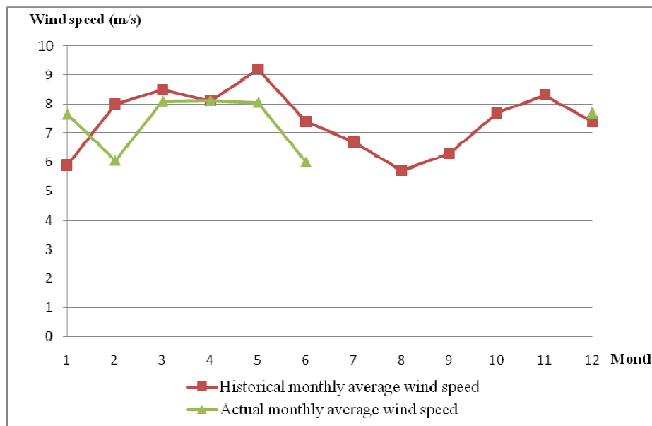
Figure 4. Comparison between the historical monthly average wind speed and the actual monthly average wind speed
