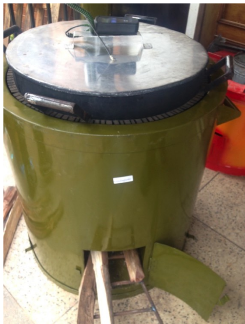
Figure 4 - UgaStove portable rocket firewood IICS for 100 litres saucepan capacity with a thermal efficiency of 35.3%
