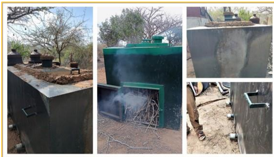
Figure 28: The various testing, modification and fabrication stages of the improved kiln including loading points and breathers during the M 8 monitoring period
