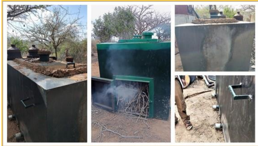
Figure 28: The various testing, modification and fabrication stages of the improved kiln including loading points and breathers during the M s monitoring period
