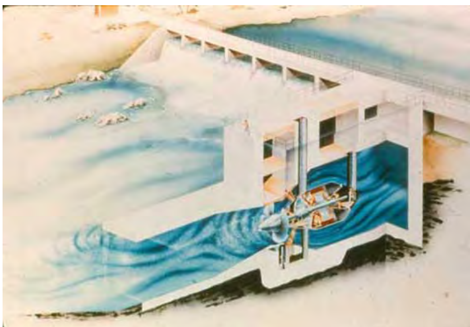
Figure 3: A representative drawing that exhibits how a bulb type Kaplan Turbine works.
