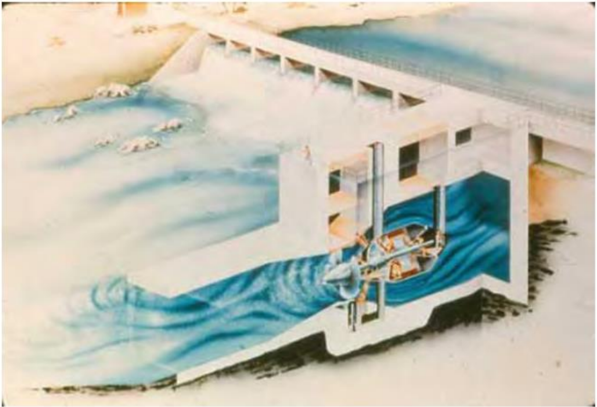
Figure 1.2. A representative drawing that exhibits how a bulb type Kaplan Turbine works.
