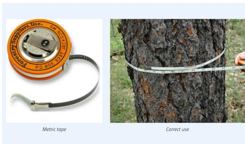
Picture 43: Measuring tape to measure the circumference at breast height
