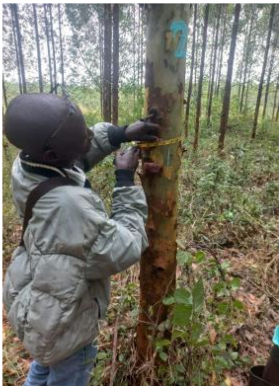
Picture 44: Measuring circumference at breast height with the measuring tape at 1.37m height
