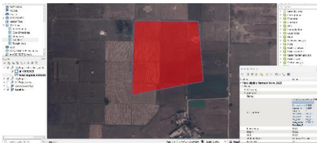
Figure 10: Improper delineation of land field
