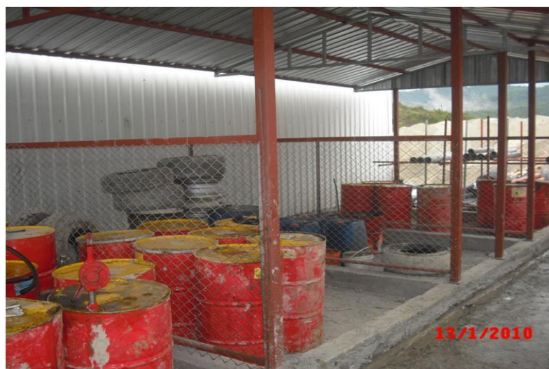
Figure 8: A scene from the chemicals that are stored in closed containers with secondary containment.
