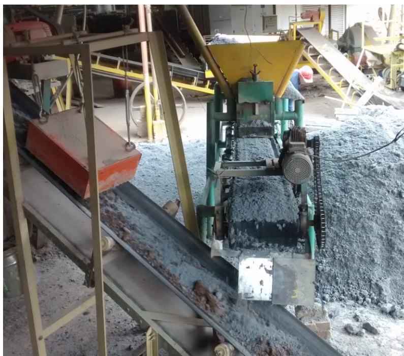
Figure 4. Pulp and paper sludge mixed with the clay for the brick production
