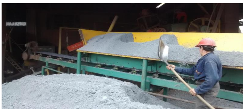
Figure 3. Pulp and paper sludge mixed with the clay for the brick production
