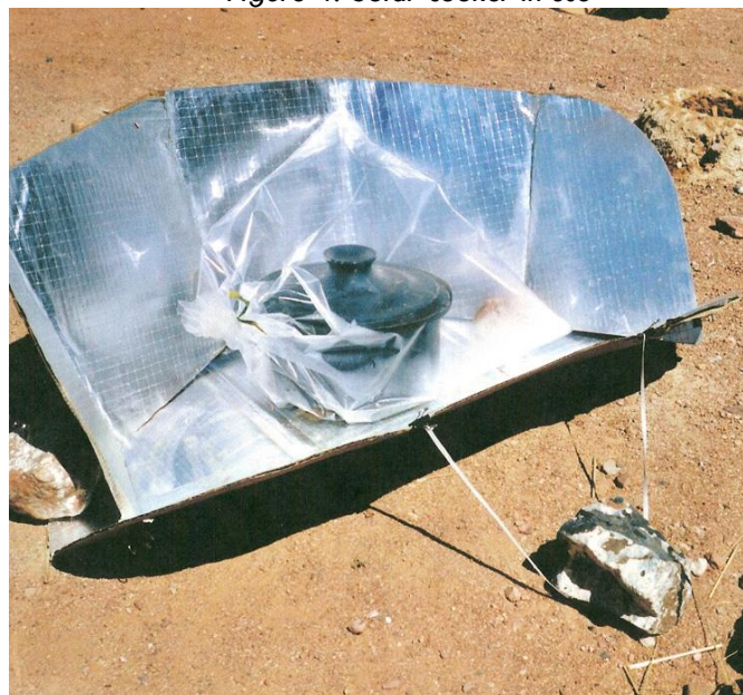
Figure 4: Solar cooker in use
