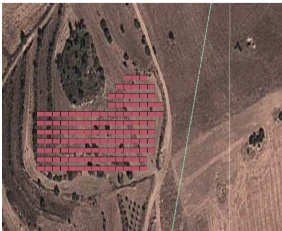
Figure 5 : Positioning of the collectors on the project site
