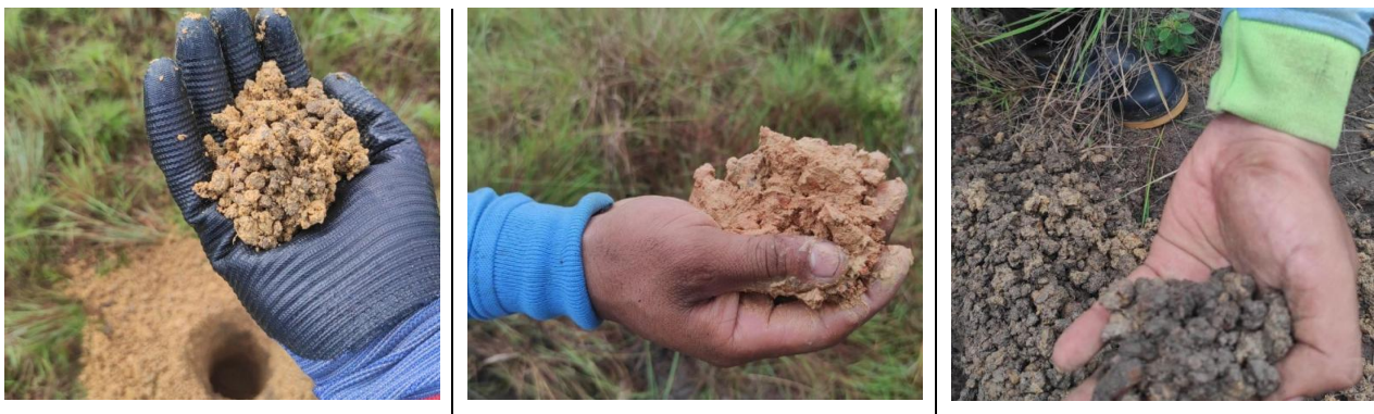
Figure 3. Identification of soil type through establishment of calicatas
